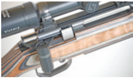
Action unlocked here we can see the rectangular lug has been lifted from its cut-out prior to bolt retraction
