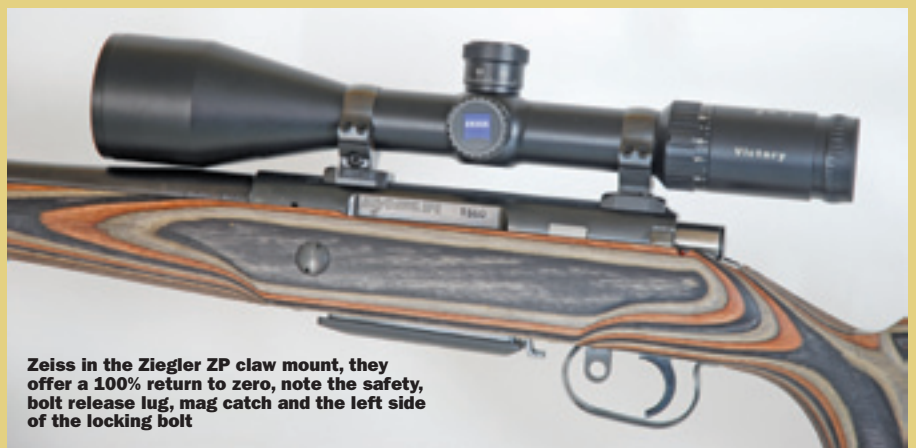
Here we see the bolt handle unlocked prior to cycling, a finger tip grip on the handle is advised, note the 17mm dovetail and the rear Ziegler ZP claw mount
